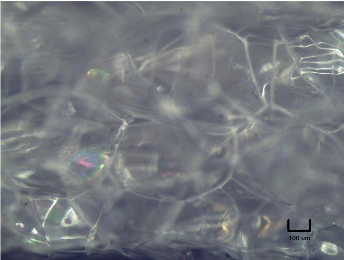
Figure 3: Scanning Electron Micrograph of Insultex. The magnification is 54X. The micrograph illustrates the cellular structure of Insultex.
