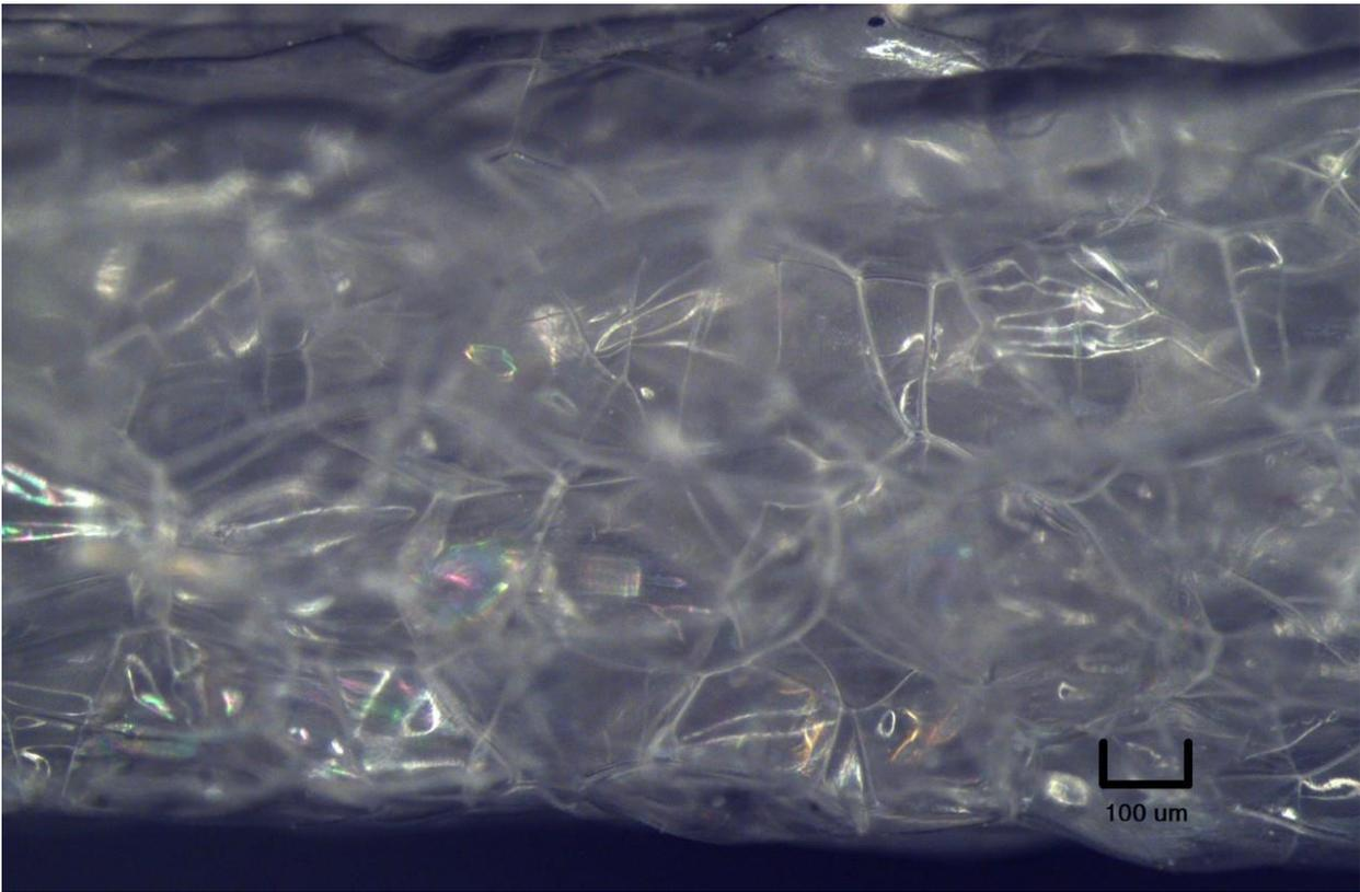
Figure 4: Scanning Electron Micrograph of the cross-section of Insultex. The magnification is 27X. The micrograph illustrates the cellular structure of Insultex.
